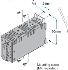
Wall mounting by using the FRK panel
