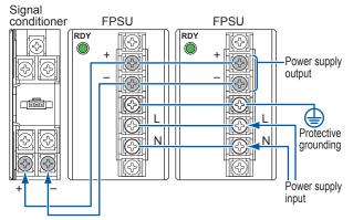
Even if one FPSU fails, the parallel connection enables the backup operation by another FPSU.
